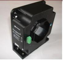
RTLT2000SH series current sensor is a closed loop device based on the measuring principle of the hall effect and null balance method, with a galvanic isolation between primary and secondary circuit, the size of primary doesn't affect test precision, no matter the location of primary in the hole of current sensor, It can really measure resolution 1000:1 and it uses for precision measurement of DC, AC and pulse current.
