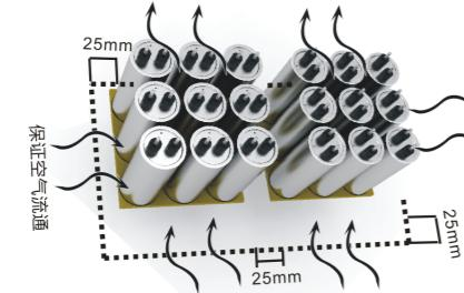
Capacitors must be installed in a well ventilated space or to ensure that no more than Specified temperature range. No matter what installation method is used, the capacitor group and the group need at least 25mm and the distance between the 25mm and the mounting plate and the metal component is at least 15mm.
