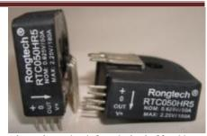
RTC50HR5 series multi-range current sensor is a closed loop device based on the principle of the hall effect and null balance method, it isolation between primary and secondary, It provides accurate electronic measurement of DC, AC or pulsed currents.
